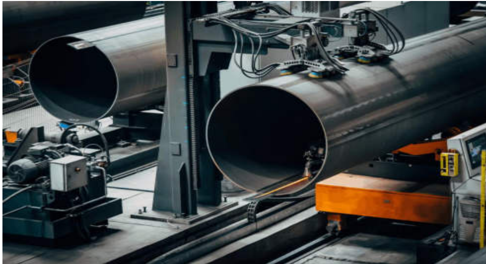
Fig.4.2.7 internal & external welding
