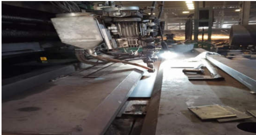
Fig.3.2.4 coil joining by saw welding
