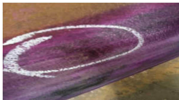
Fig.5.2.4 DPT Test (pitting is marked)
