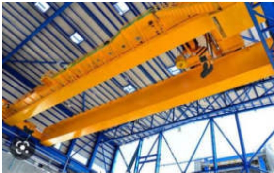
Fig: 2.20 Overhead Crane
