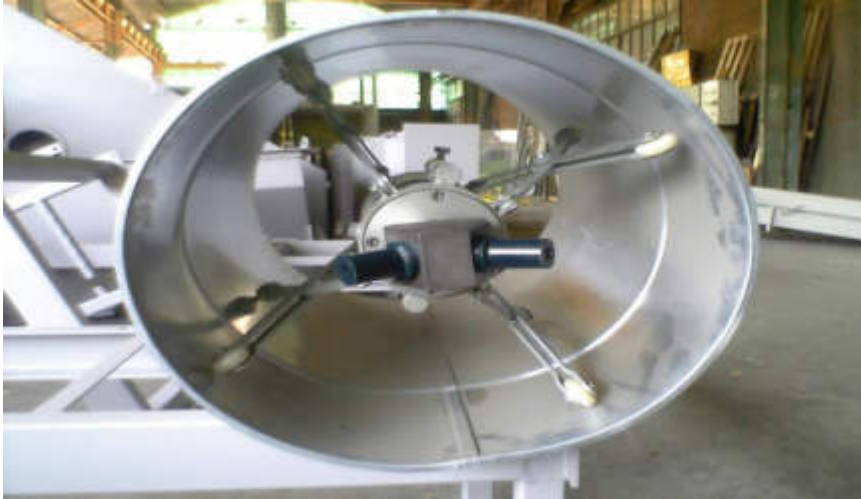
Fig.7.3.6 internal paint spray
