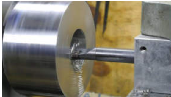
Fig: 7.3 Boaring Operation
