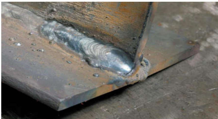
Fig.6.1.6 Spatters in welding
