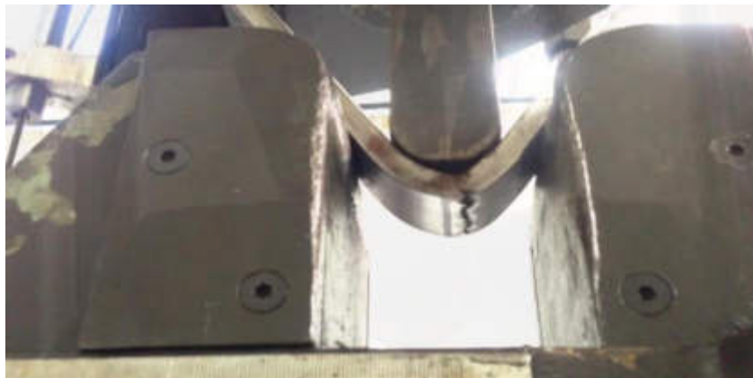
Fig.5.1.2 Guided bend test
