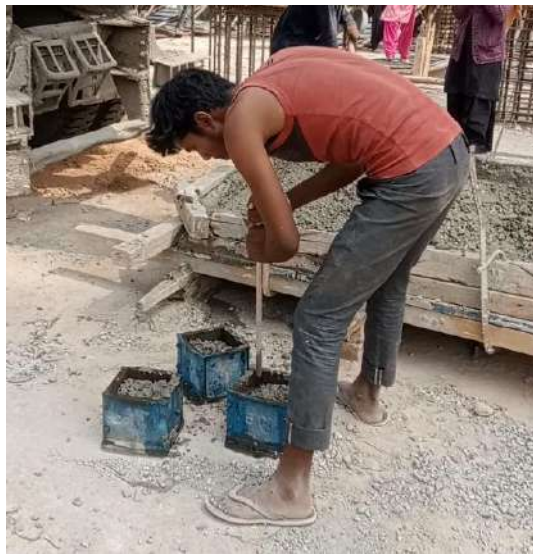
Fig: 12.3 Cube casting
