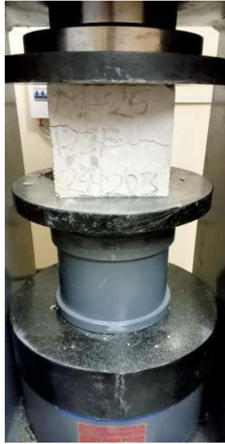
Fig: 13.9 Cube testing
